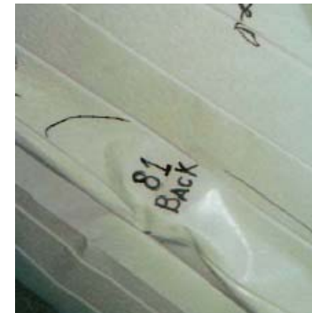
Inside surface bent but not penetrated
