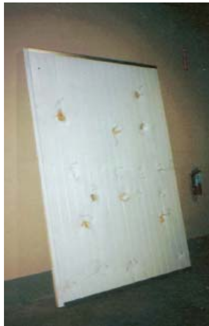
Localized wall penetration occurred at 234% of Dade County test specification.
